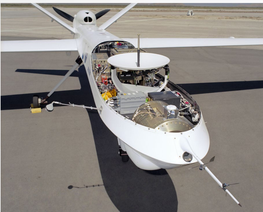
Existing airborne sat-com solutions use gimbal stabilised, high gain antennas. Small panel antennas with electronic beam steering will allow integration into smaller vehicles, with higher bandwidths and lower costs. (Photo: NASA)
